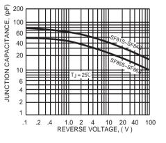
FIG. 2 - TYPICAL REVERSE CHARACTERISTICS
